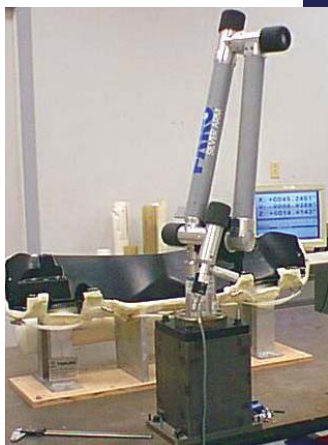
Faro Arm and 3D inspection software compare finished parts to their CAD models.
